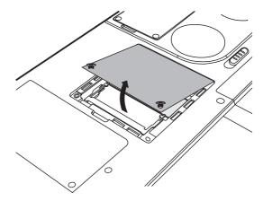
Removing the memory module socket cover
